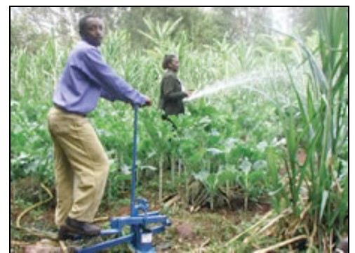
African farmers use one of KickStart's foot-operated irrigation pumps to water crops. This simple and
